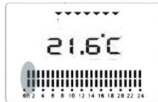
Use the +/- keys to advance through the hours, from 0 – 24. The hour will flash to indicate that it is currently selected. When an hour is selected, use the ☼, ☺, ☻ and ⏹ keys to set a heat level for that hour.
