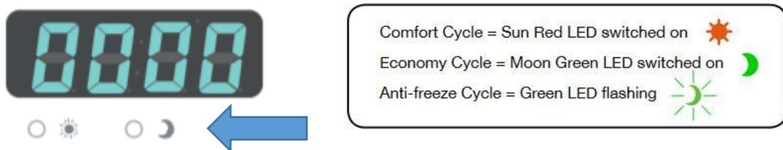
So, for example, if you want to have your heater in Economy mode at this time, press the up/down arrows until the Moon LED is on (and not flashing). Then press OK to confirm the setting for this hour. The screen will then advance to the next hour.
