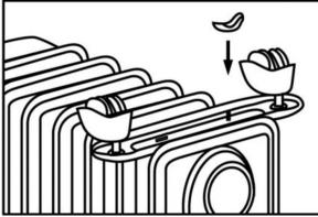
Figure 1: Attaching castors to heater body
