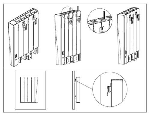
Figure 5 | Secure unit with locking screws
