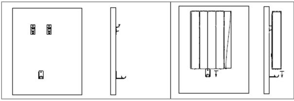
Figure 4 | Mounting radiator on wall
