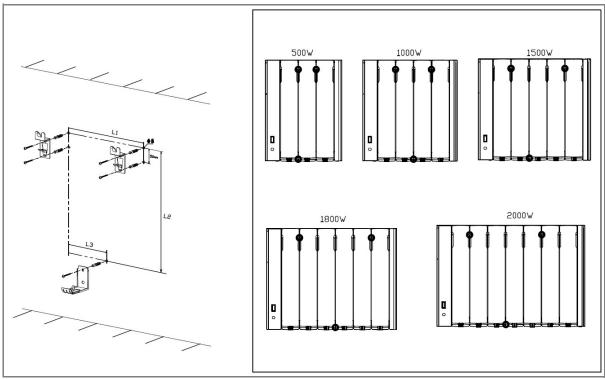
Figure 3 | Bracket positions on the radiator and wall
