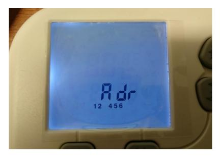
After a few seconds the thermostat will return to the main screen. Plug in the receiver, and get the thermostat to resend the signal by turning it to a low temperature, waiting 30 seconds, and turning it to a high temperature. The receiver will switch on. If it doesn't switch on, there may be interference, please start again trying a new code.
